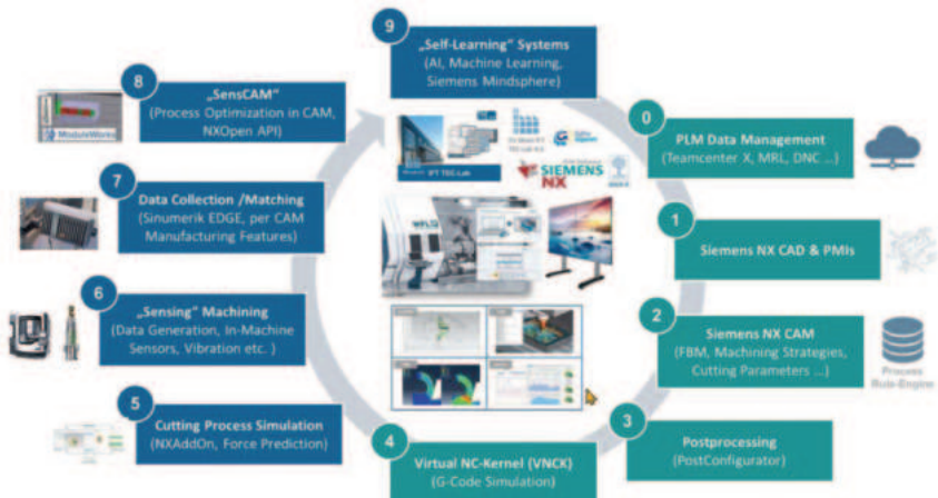
Figure 6: Overview closed-loop approach at TU Wien (IFT).
