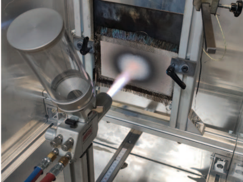
Figure 4: Ballistic and thermal protection test of flexible CMC.
