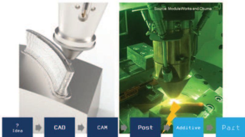
Figure 1: Process chain in additive manufacturing.
